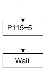
P115=5 Controller Optimization Alarm message "A080" will appear, and a start command must be issued within 20 seconds to perform the test, otherwise P115 will unset.
